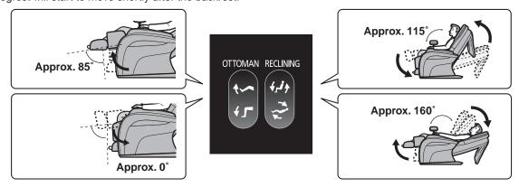
\*The reclining operation is a function that adjusts the angle of the backrest and legrest. Avoid using it for any other purposes, such as continuous up/down operation etc.
